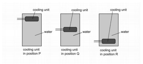
In order to cool all the water as quickly as possible to  $5\,^{\circ}$ C, in which position should the cooling unit be fitted, and should the outside of the container be dull black or shiny?
