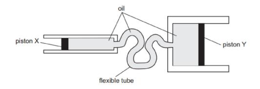
When the driver presses on the brake pedal, a force is exerted on piston X. The pressure produced in the oil by this force is transmitted through the oil so that it causes a force to act on piston Y. This presses the brakes against the moving parts.
