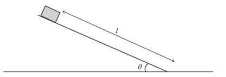
The block experiences a friction force of  $kW\sin\theta$ , where W is the weight of the block and k is a constant.
