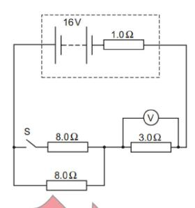
Which line in the table gives the voltmeter readings when switch S is in its open and closed states?
