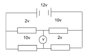
So, reading on voltmeter is 10v - 2v = 8vAnswer is E.
