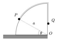
The diagram shows two particles, P and Q, connected by a light inextensible string which passes over a smooth block fixed to a horizontal table. The cross-section of the block is a quarter circle with centre O, which is at the edge of the table, and radius a. The angle between OP and the table is  $\theta$ . The masses of P and Q are m and M, respectively, where m < M.
