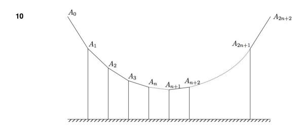
The above diagram represents a suspension bridge. A heavy uniform horizontal roadway is attached by vertical struts to a light flexible chain at points  $A_1=(x_1,y_1), A_2=(x_2,y_2),\ldots,$   $A_{2n+1}=(x_{2n+1},y_{2n+1}),$  where the coordinates are referred to horizontal and vertically upward axes Ox,Oy. The chain is fixed to external supports at points
