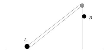
The diagram shows a small railway wagon A of mass m standing at the bottom of a smooth railway track of length d inclined at an angle  $\theta$  to the horizontal. A light inextensible string, also of length d, is connected to the wagon and passes over a light frictionless pulley at the top of the incline. On the other end of the string is a ball B of mass M which hangs freely. The system is initially at rest and is then released.
