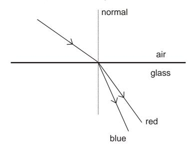
Red light travels at speed c in air, but only 2c/3 in glass. Red light has a wavelength of  $\lambda$  in air.
