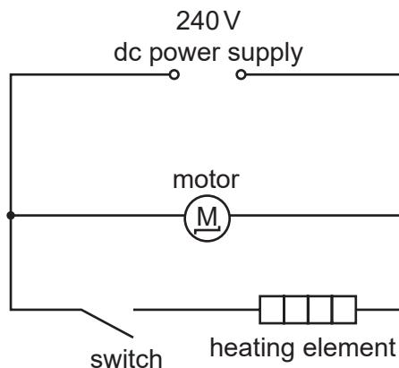
At first, the switch is open and the current in the motor is 0.40A.
