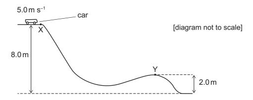
How much energy is transferred in overcoming resistive forces as the car travels from X to Y? (The gravitational field strength g is  $10 \,\mathrm{N\,kg^{-1}}$ .)
