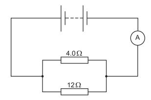
The power dissipated in the  $12\Omega$  resistor is 12W.
