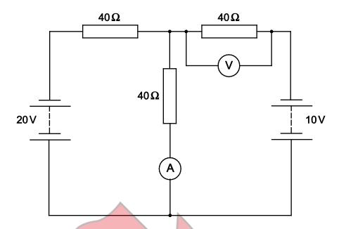
What are the readings on the ammeter and the voltmeter?
